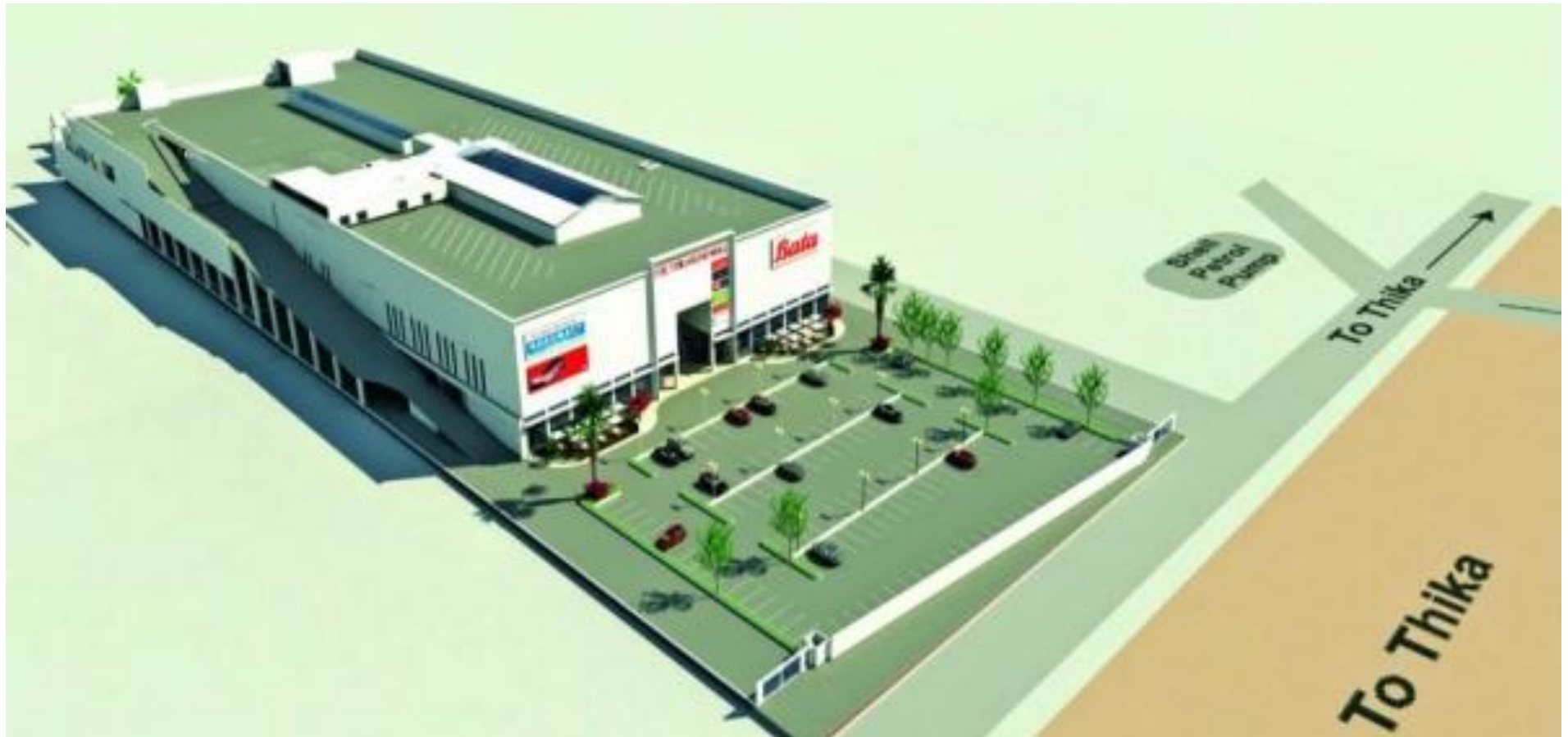
Fig 4.61: A model showing both the layouts of the front and roof-top parking lots at Thika Road Mall and their servicing from the Thika Super-Highway. The ramp to the roof can be seen on the left side of the model. Source; Studio Infinity Architects
